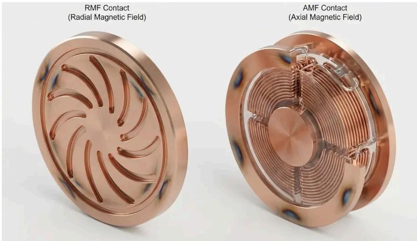
At high fault currents ( $>10\text{kA}$ ), the arc's own magnetic field causes it to constrict into a tight, incredibly hot column that can destroy contacts. Engineers use magnetic fields to control this.
