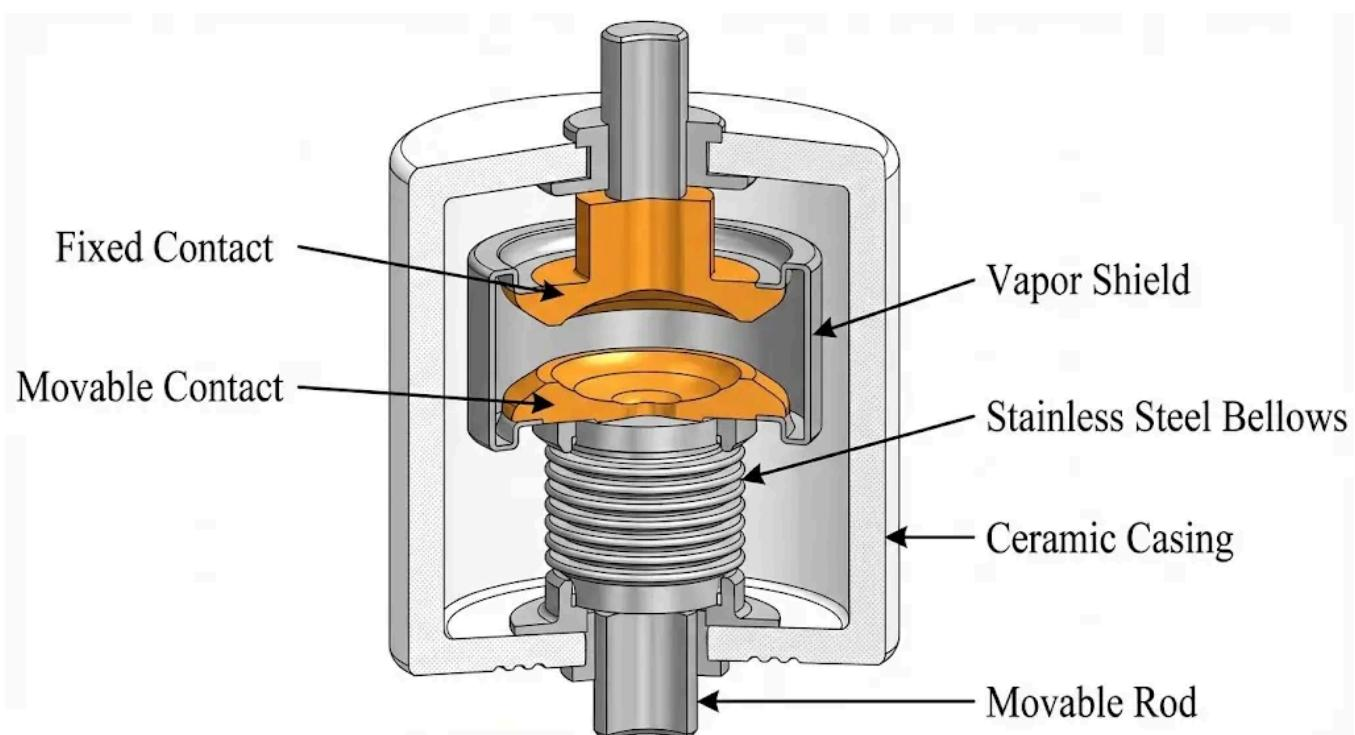
A vacuum interrupter is a complex assembly of high-purity materials joined by advanced vacuum furnace brazing.
